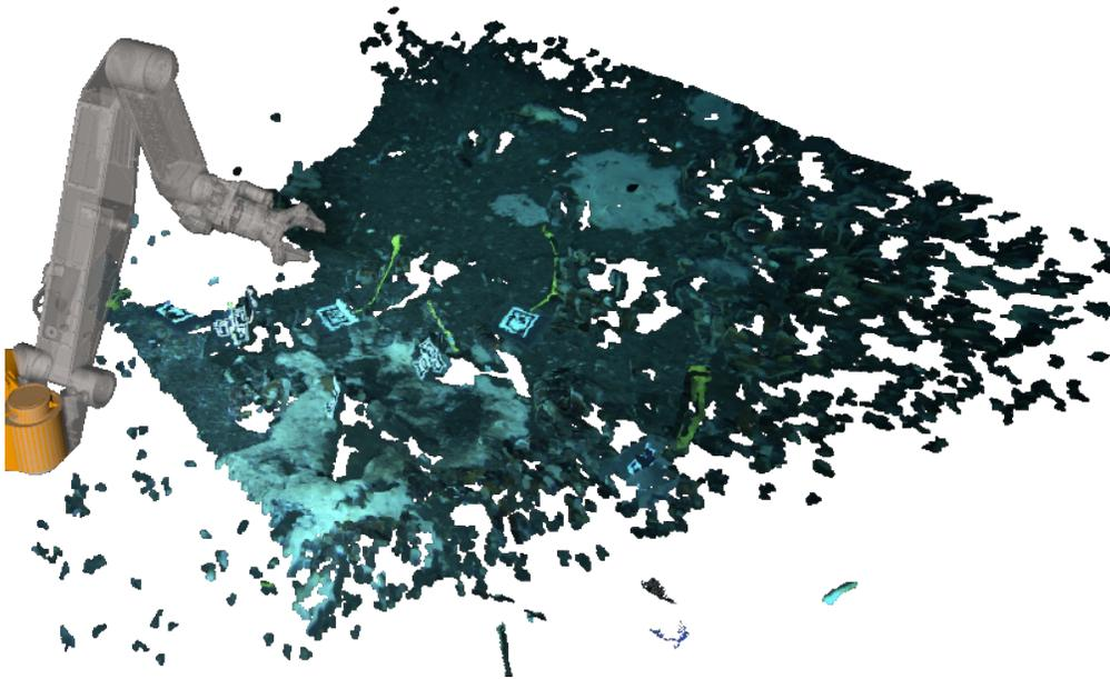
Figure 10: The vision system was integrated on the *SuBastian* ROV operated by Schmidt Ocean Institute, where we demonstrated real-time visualization of the planning scene with a Schilling Titan-4 manipulator and the projected stereo point clouds. This also demonstrates the flexibility of the system to be integrated with different vehicles and manipulators.
