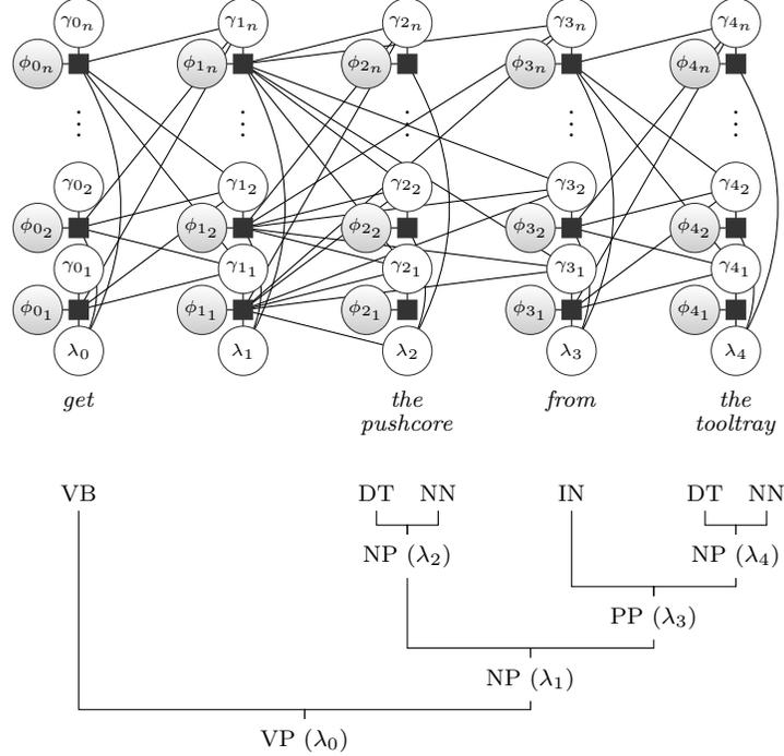
Figure 18: A visualization of (top) the DCG factor graph for the expression “get the pushcore from the tooltray” aligned with (bottom) the associated parse tree. Shaded nodes denote observed random variables, while those rendered in white are latent.
