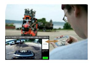
Fig. 1. The supervisor commands the forklift to lift a pallet from a truck, by circling the pallet on the robot's-eye-view displayed on the tablet interface (inset). The tablet also interprets simple spoken commands to summon the forklift to various task areas within the warehouse.
