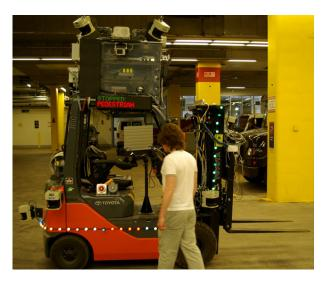
Fig. 9. The forklift detects an approaching pedestrian and pauses. Colored lights skirting the vehicle indicate the proximity of close objects (red to green lights map range from close to far). The LED signs display the reason for pausing
