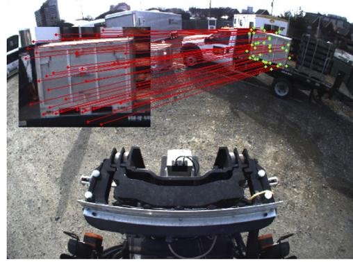
Figure 4. A visualization of an object being matched to an appearance model (inset) derived from the user’s stylus gesture. Red lines denote correspondence between SIFT features within the initial view (red) to those on the object in the scene (green).
