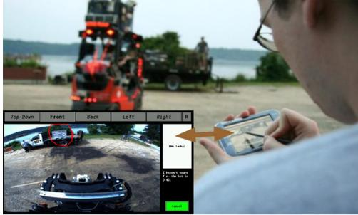
Figure 1. The robotic forklift manipulates and transports cargo under the direction of a human supervisor who uses speech and stylus gestures on a hand-held tablet to convey commands.
